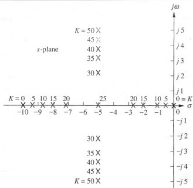
As the gain increases, the closed loop pole which is at -10 for  $K=0$  moves to the right and the pole which is at 0 for  $K=0$  moves to the left. They meet at -5 and then break away from the real axis and move into the complex plane. If we replace the individual pole locations with solid lines, we obtain the root locus plot for the system.
